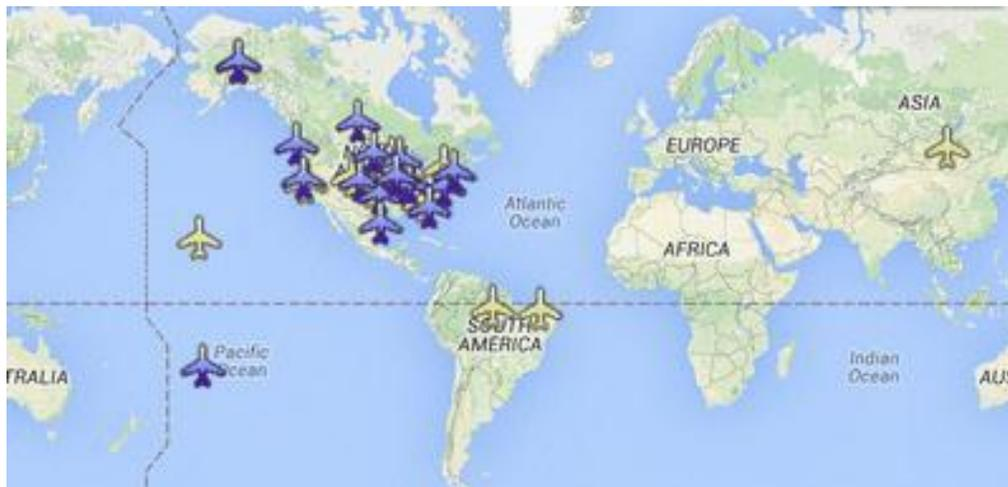
Figure 3. Location of air-based program measurement sites. Aircraft in yellow represent inactive sites.
